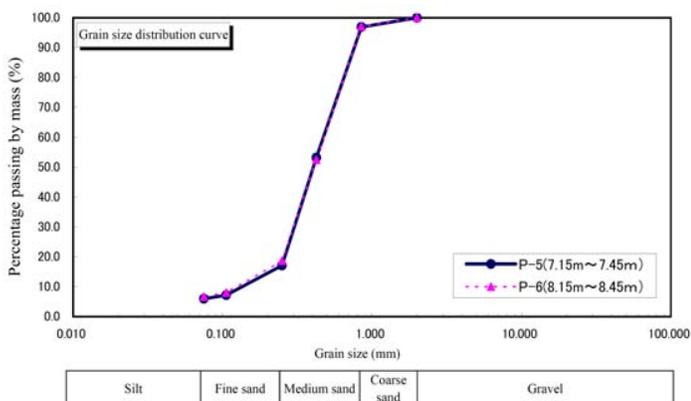
Fig.21 Results of liquefaction layer grain size analysis(GL-7~9m)
