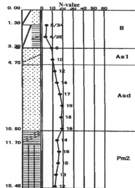
Fig.20 Results of standard penetration test
