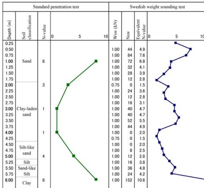
Fig.11 Results of SPT test and SWS test
