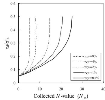
Fig. 10. Relation between  $N_a$ ,  $\gamma_{cy}$ , and  $\tau_d/\sigma'_z$
